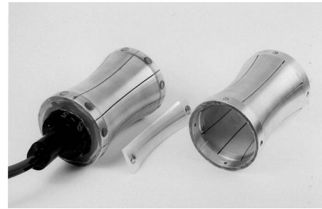
FIG. 2. The DRDC Atlantic class I barrel-stave flextensional transducer on the left has eight concave aluminum staves that are attached to an octagonal mild steel end plate. The slotted-shell with a circular cross-section (left) can also be used as the radiating shell (see Ref. 18). Photograph by H. Merklinger, DRDC Atlantic, 2002.
