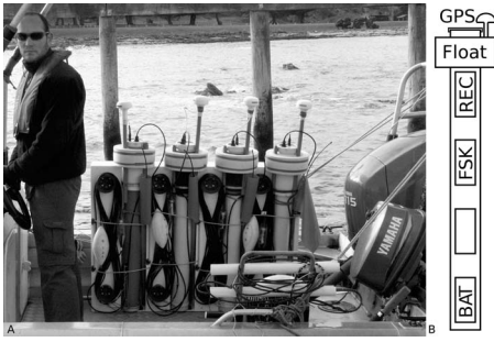
FIG. 1. (A) Photograph of 4 buoys and boat-based array ready for deployment from the research vessel. (B) Buoy schematic showing arrangement of the Microtrack recorder (REC), GPS receiver, FSK modulation electronics, and power supply (BAT).
