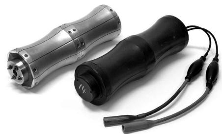
FIG. 3. Two DRDC Atlantic Class III dual-shell barrel-stave flextensional transducers. Note that the transducer on the right is sealed with a neoprene rubber boot, which is required on all barrel-stave designs to prevent seawater ingress. Photograph by Donald Glencross, DRDC Atlantic, 2004.
