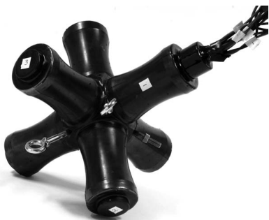
FIG. 5. The flextensional cluster transducer protected by a neoprene rubber boot. Photograph by Donald Glencross, DRDC Atlantic, 2008.
